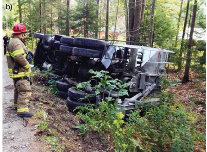
Fig. 3(a) and 3(b): A driver mentally unfit to operate a truck took a turn too quickly and rolled over fully loaded mobile mixer. The body was able to be repaired but the truck was totaled
