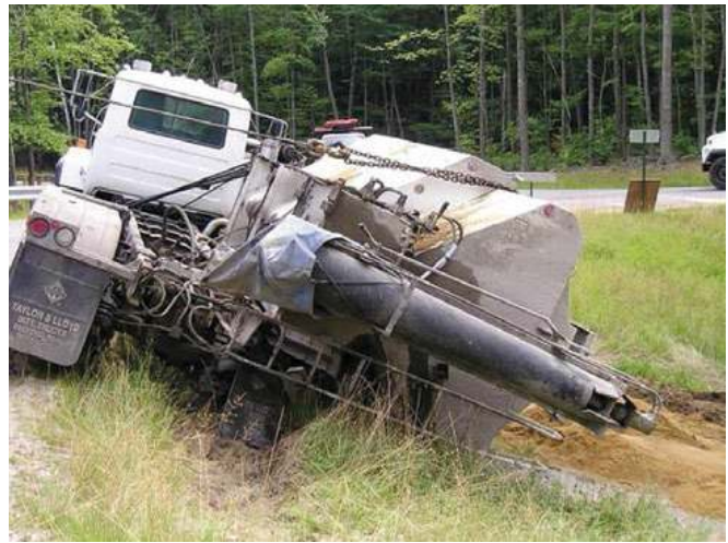
Fig. 2: An example of why vehicle inspections and knowing your truck are so important. This body broke loose from the frame of the truck and tipped over
