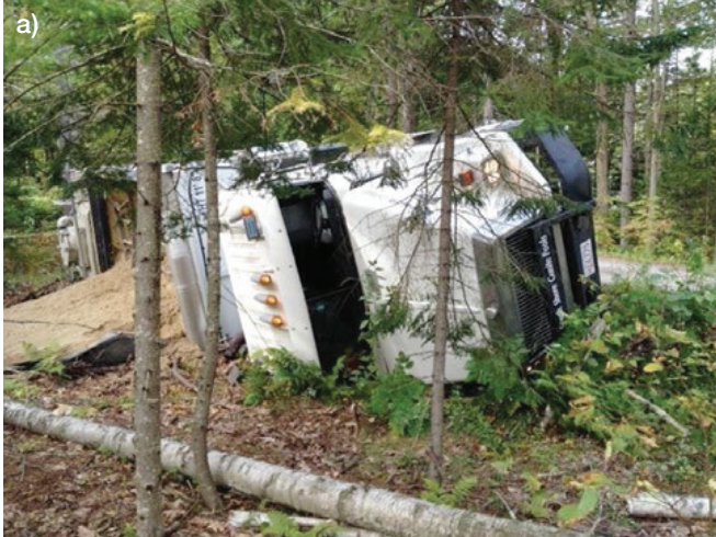
Fig. 3(a) and 3(b): A driver mentally unfit to operate a truck took a turn too quickly and rolled over fully loaded mobile mixer. The body was able to be repaired but the truck was totaled
